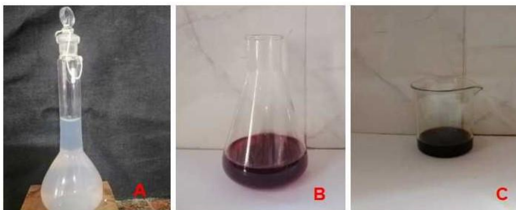
Fig. 1: (A) Solution of Silver Nitrate before, (B) after the addition of flower extract, and (C) silver nanoparticle formation after three hours.
