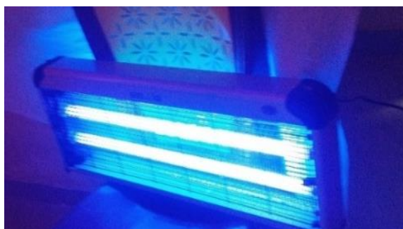
Fig. 2: Box type light trap used to capture moths.
